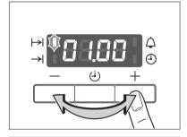
After approx. 5 seconds the display returns to showing the current time. The function indicator Cook time → lights up.
